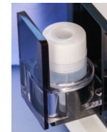
Figure 2: Close-up of a PythoN i channel with a tissue dissociation tube.
